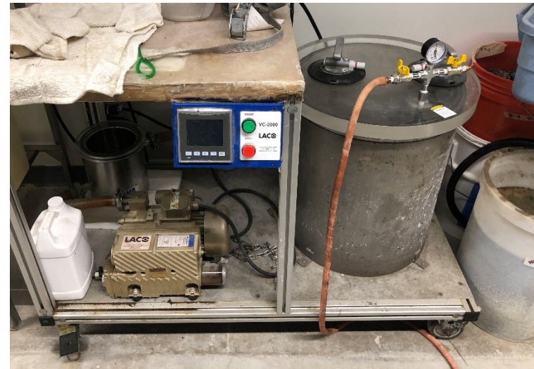
Concrete sample saturation system
