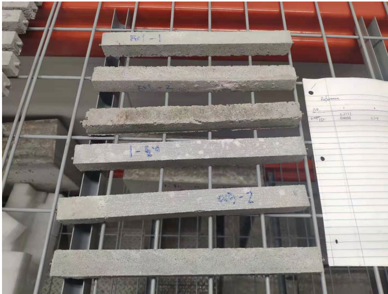
Samples and setup for drying shrinkage measurement
