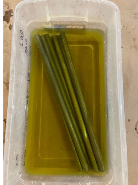
Rebar washed by the sulfuric acid (get rid of rust and coating oil)
