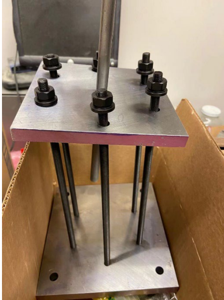
Setup for rebar pull-off
