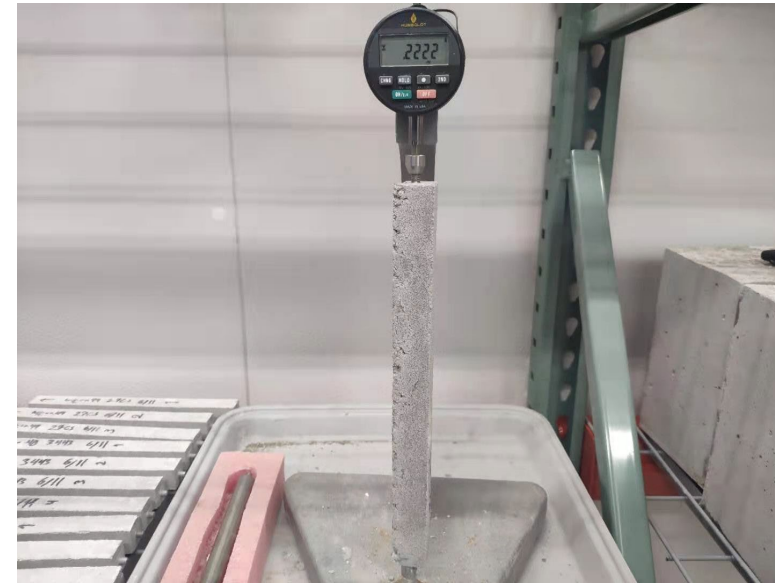
Samples and setup for drying shrinkage measurement
