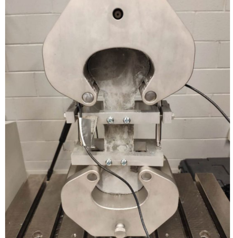
Dog-bone specimen under tensile loading
